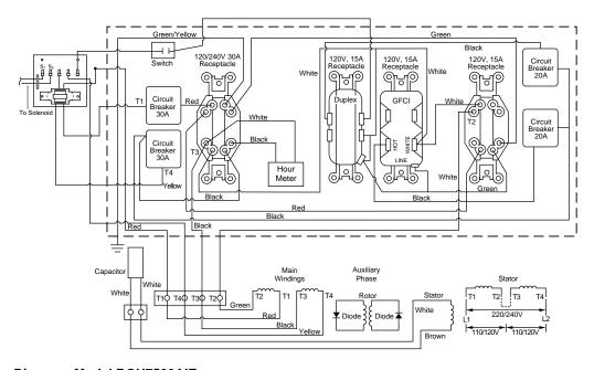
Figure 34 - Wiring Diagram, Model RGH7500AIE
